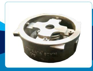
KAVAATA Non-Slam Check Valves are made from Investment Castings, designed and manufactured as per BS7438/ASME 16.34. The valve can be supplied in sizes like 1/2" to 4". The common materials of construction are ASTM A216 Gr WCB (CS), ASTM A351 Gr CF8 (SS304) and ASTM A351 Gr CF8M (SS316).
